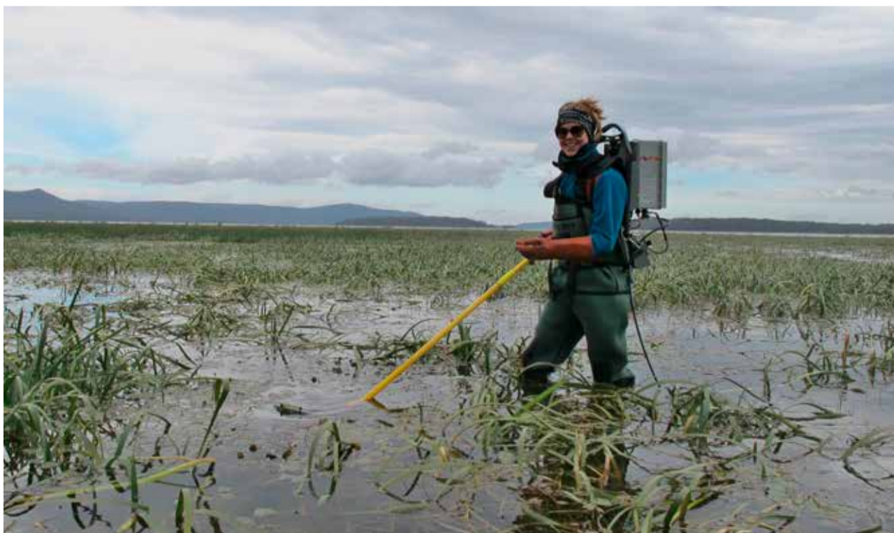
Backpack shocking for invasive European carp in the marshes of Lake Sorrell, Tasmania, Australia.
