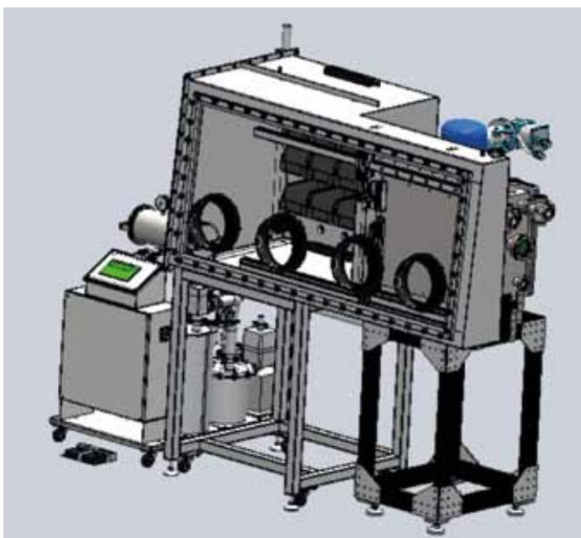
Figure 3: LC tech glovebox with our in-house integrated vacuum chamber designed to further develop the project.
