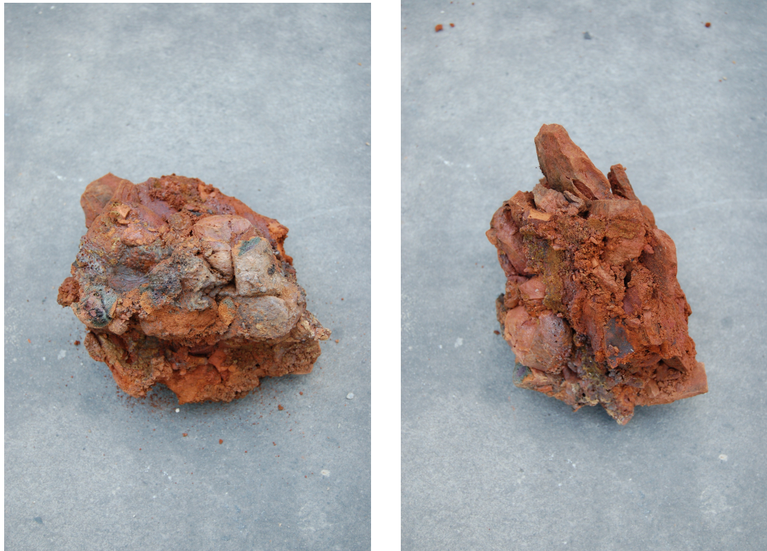
Fig. 8: a piece of vitrified material / flow slag, original dimensions c. 15x10x10 cm
