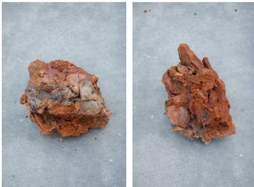
Figure 8: a piece of vitrified material / flow slag, original dimensions c. 15X10x10 cm.
