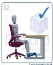
Set the chair position / height as described. Use a footrest if the feet do not touch the ground. Height-adjustable chair arms provide additional support for the upper body when not keying. If the armrests restrict desk access, ask if they can be removed.
