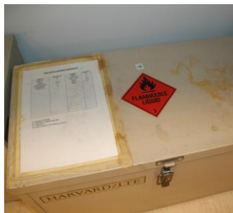
Storage Unit marked to show contents & hazards
