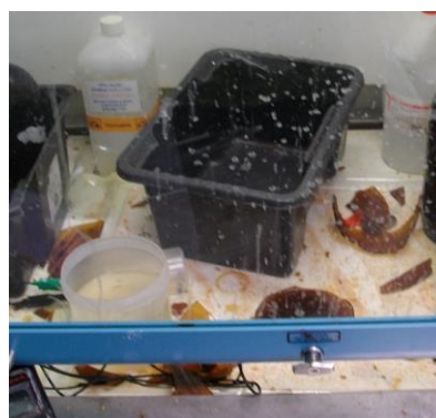
Winchester jar exploded due to severe over pressure caused by rapid gas generation
