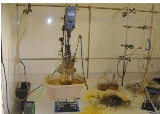
Fire caused by a runaway reaction
