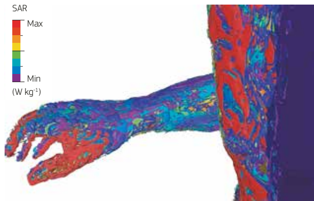
Figure D10 — The determination of dose quantities, in this case the SAR in the hand and torso from exposure to an unshielded cable, for direct comparison with the ELVs. The Directive recommends this approach to demonstrate compliance for very localised electromagnetic field sources within a few centimetres of the body
