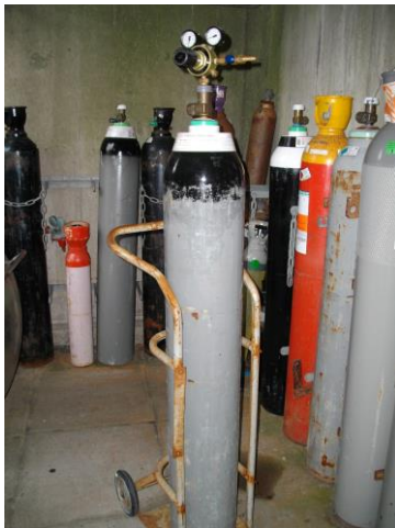
Safety chain not in place, regulator still connected
