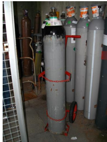
Both safety chains in place, regulator removed
