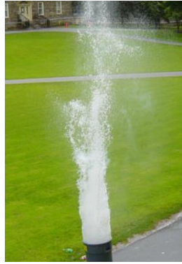
Explosion - caused by boiling liquid nitrogen
