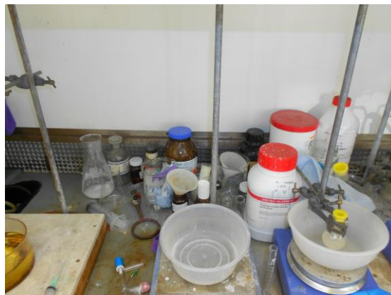
Poor Housekeeping: Unlabelled items, spills not cleaned up, general mess and items too close to the lower vent grill restricting airflow
