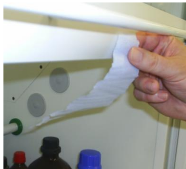
Direction of paper movement shows the air is drawn into the Fume Hood
