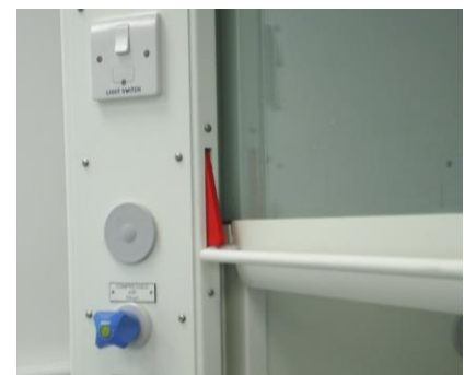
Red tab indicates the Safe Working Limit. Try to work with the sash lower if possible
