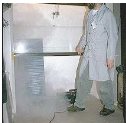
The difference in capture efficiency if the sash is lowered properly
