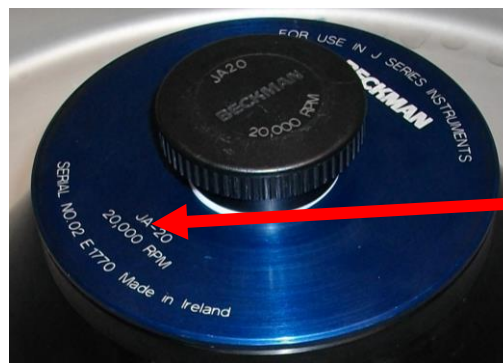
Maximum rotor speed of 20,000 RPM
