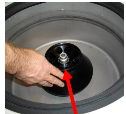
Spin rotor to check pins are located and rotor moves freely
