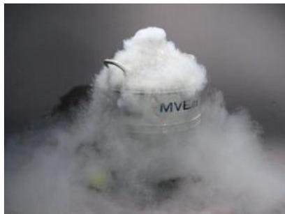
Liquid nitrogen is an inert, colourless and odourless liquid, similar in appearance to water and which because of its coldness and ability to rapidly cool and freeze items, is widely used as a coolant in laboratories.
