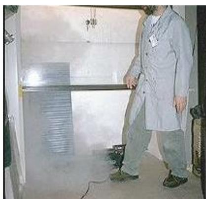
The difference in capture efficiency if the sash is lowered properly
