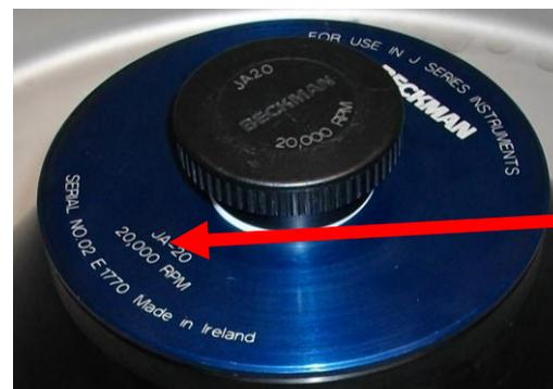
Maximum rotor speed of 20,000 RPM
