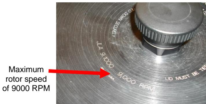
Maximum rotor speed of 9000 RPM
