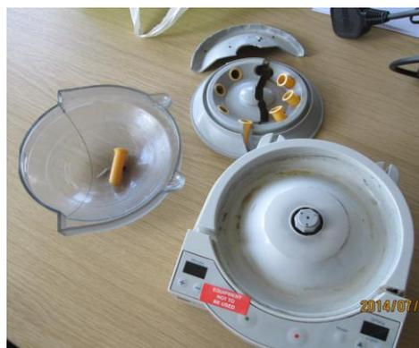
Structural failure, possibly due to not being cleaned over time causing integrity to deteriorate
