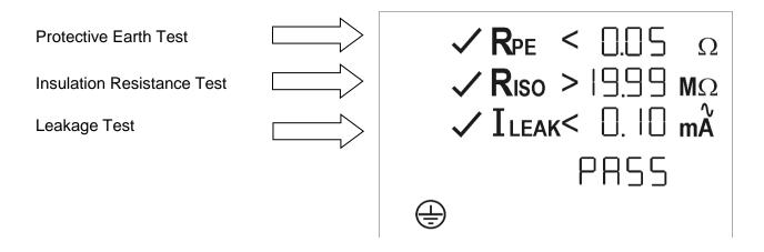
As the Insulation Test will probably give an *apparent fail* due to the surge protection, you need to check the Leakage Reading is below the required limits (as per PrimeTest 100 Factory Set Pass / Fail Limits):
