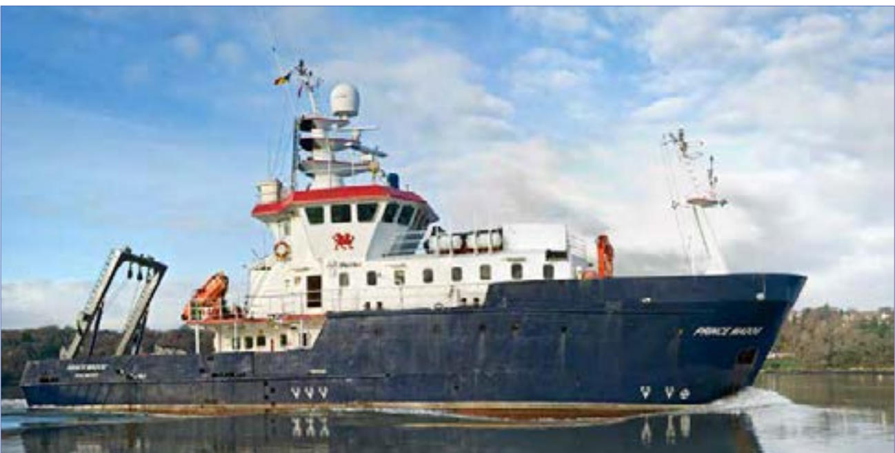
Figure 3 The second RV Prince Madog . In 1999, as a result of a Joint Infrastructure Fund bid led by Ed Hill (then at Bangor) funding became available for a new ship, which came into service in 2001. Built by Scheswerf Visser BV, the new Prince Madog (390 tonnes, 34.9 m in length) arrived in Menai Bridge in summer 2001. She is more spacious and stable than her predecessor, and has capacity for 11 scientists and an endurance of 10 days. (Photo: School of Ocean Sciences, Bangor University)
