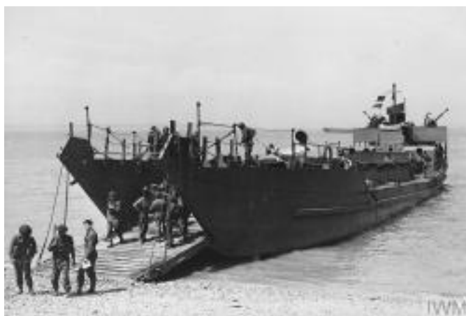
LCT 326 was a Mk III 'Landing Craft Tank' designed to land armoured vehicles during amphibious operations. Image courtesy Imperial War Museum
