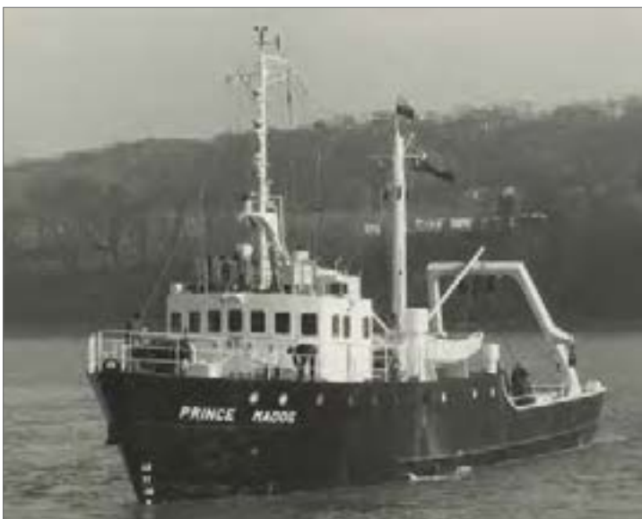
Figure 1 The original RV Prince Madog approaching Menai Bridge pier in 1968. The 185-tonne, 28.7-m research vessel, built on the Isle of Man, could accommodate eight scientists and had an endurance of seven days. She was named after the Welsh Prince who, legend says, set sail in 1170 on a westerly course, eventually reaching North America, where he founded a Welsh-speaking tribe.
