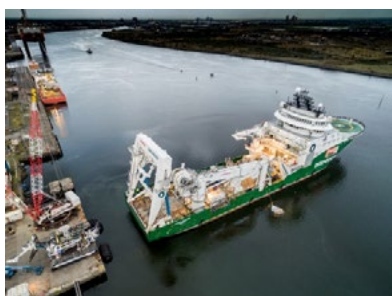
Burial machine load-out onto the DeepOcean construction vessel Havila Phoenix on the River Tees, ahead of installation operations on the Nemo Link
