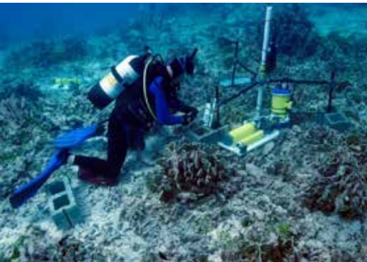
Figure 5 and 6: Deployment of BEAMS (Benthic Ecosystem and Acidification Monitoring System) and ARMS (Autonomous Reef Monitoring Structures). (Fig 5 Rob Dunbar)
