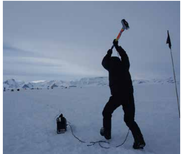
Seismic survey on Larsen C Ice Shelf
