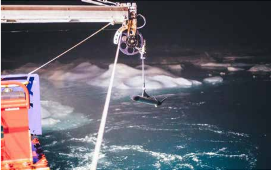
Researchers deploy a Fast CTD developed at Scripps Oceanography during the 2018 SODA cruise in the Arctic Ocean.
